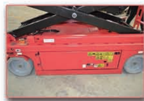
Innovated Pothole Protection
