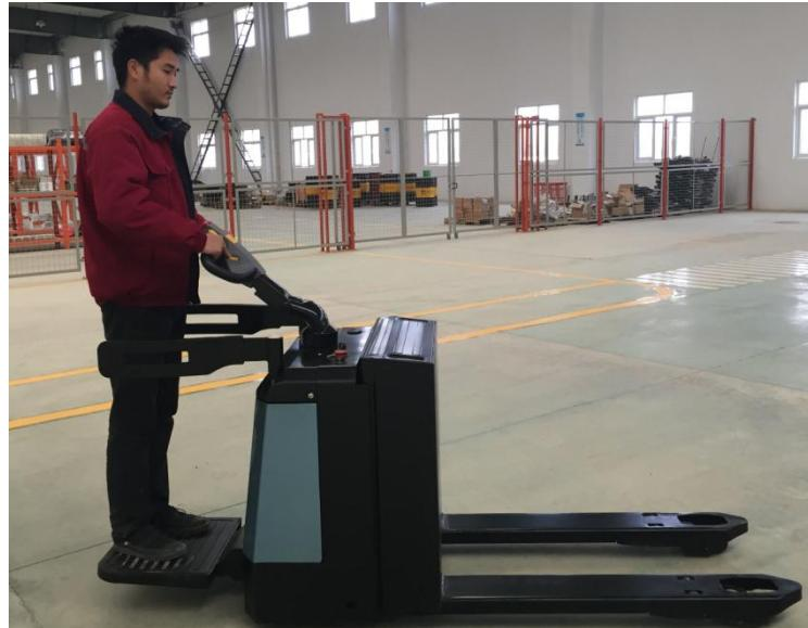
➤ Fold the platform and pedestrian drive, automatic switch to low-speed walking mode
