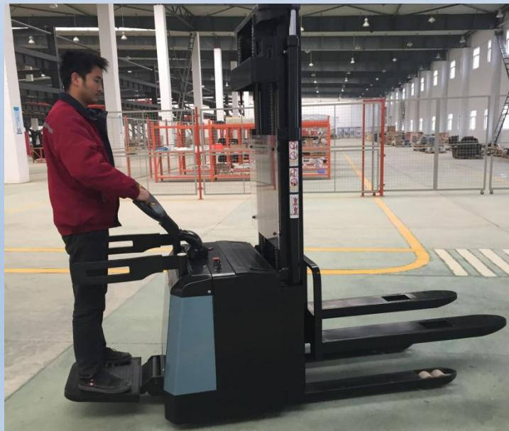
➤ Fold the platform and pedestrian drive, automatic switch to low-speed walking mode
