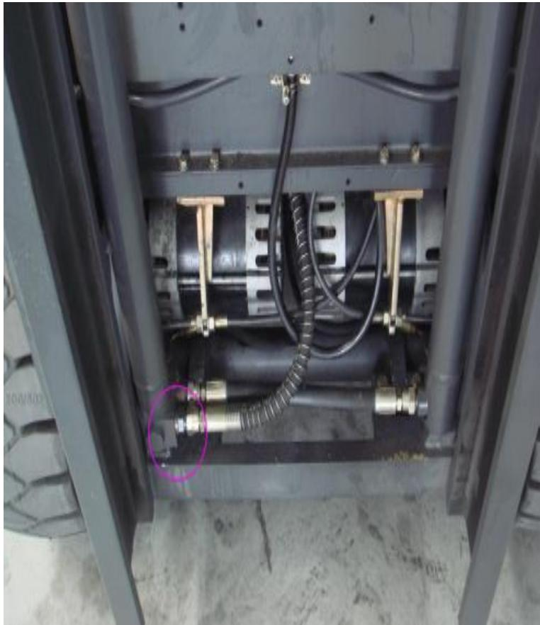
Front dual AC motor traction system
