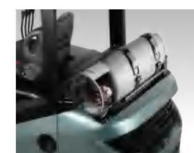
RY Gasoline/LPG forklift can be easily installed and removed in one minute. This ergonomic designed gas bracket is standard in each Gasoline/LPG forklift.
