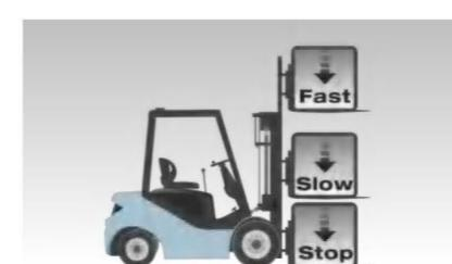
With intelligently declining buffer sensor on the two ends of the cylinder, the falling speed of the fork slows down automatically before it is 10cm from the ground, and the lifting speed to the top also slows down to avoid quick hit on the top, it super increases the safety of the goods and forklifts.
