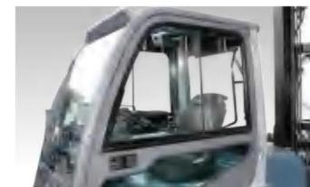
Because of the new shaped tube material applied to the overhead guard, the cabin can be removable easily. With full glass cabin and less plastic design, the operator can wide view all surroundings easily.
