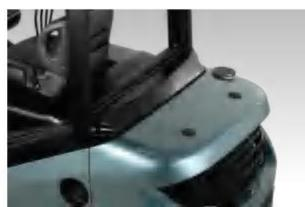
Unique design of the radiator assembly, the counter weight is not need to be dismantled when replacing new radiator. It is easy to maintain and replace the radiator.
